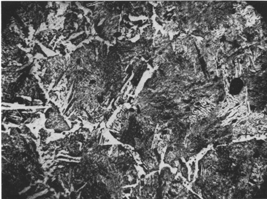
Figure 4 Micro-section of reinforced layer. Sodium Benzoic etch ( \times 1500 ).
